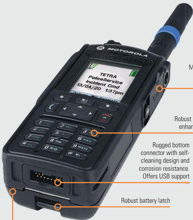
Motorola GAI rugged side connector for audio accessories.
