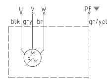
Figure 6: Three phase wiring
