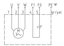
Figure 7: Three phase wiring with temperature limiter
