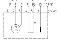
Figure 11: Single phase wiring with temperature limiter and DI
