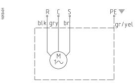
Figure 9: Single phase wiring
