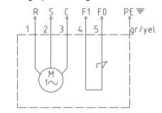
Figure 10: Single phase wiring with temperature limiter
