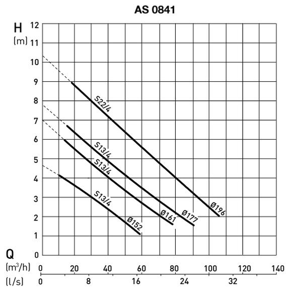
H = Total Head; Q = Discharge Volume. Curves to ISO 9906 (60 Hz available on request). N.B. please use the ABSEL program to validate pump selection.
