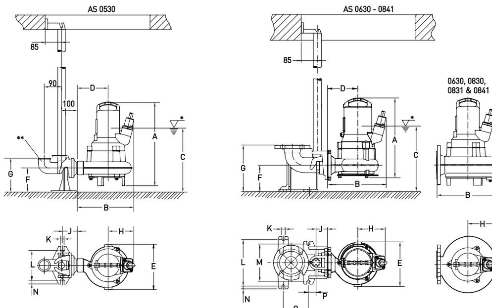
\* Lowest switch-off level; minimum switch-on level must be at least 100 mm higher.
