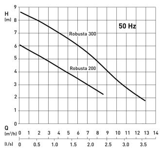
H = Total head; Q = Discharge volume Curves to ISO 9906 (60 Hz available on request)
