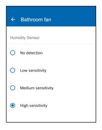
Select sensitivity of the humidity sensor. This adjusts the amount of humidity required to activate the function. Then you can use the sliding scale to increase or decrease the air moved in the function.
