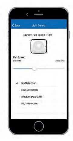
11. Select the **Sensor** function in the Function menu to customise the Fan Speed on this setting between 800 and 2400 RPM.
