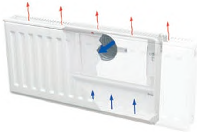
Easy-Vent installed on the wall behind the radiator (in cross-section). The filtered and pre-heated fresh air is supplied to the room at the radiator's upper edge.
