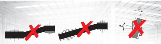
Axial misalignment of pulleys
