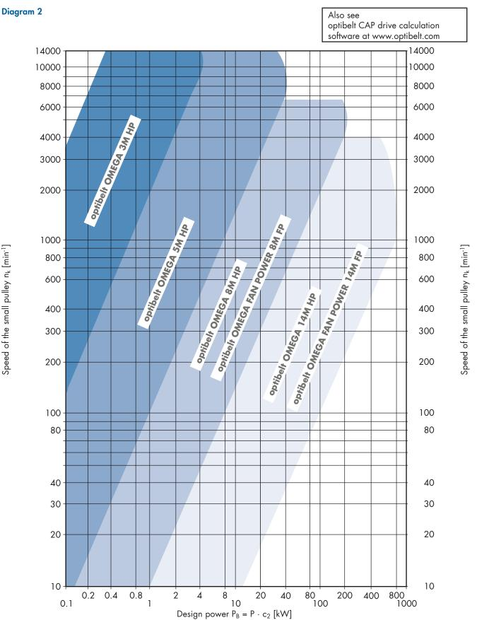
Speed of the small pulley  $n_k$  [min<sup>-1</sup>]
